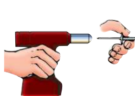
1 Insert rivet mandrel in rivet setting tool.
